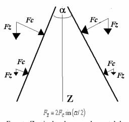
Fig.1. A projection of the force Fc onto Z axis develops an elemental thrust
