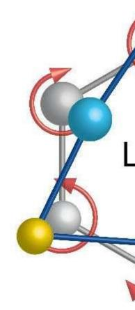
This diagram maps out atomic motion in separate phonon modes. At left ("LO" represents a longitudinal optical mode), selenium atoms exhibit a clockwise rotation while tungsten atoms stand still. At right ("LA" represents a longitudinal ...<u>more</u>
