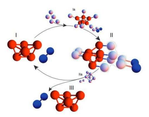
Self-Replicating Sphere Clusters: According to new research at Harvard, coating the surfaces of microspheres can cause them to spontaneously assemble into a chosen structure, such as a polytetrahedron (red), which then triggers nearby spheres into forming an identical structure.
