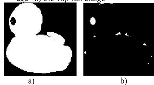
Fig.8: Applying the Bottom-hat filter: a) the Original binary image b) Bottom-hat filter image
