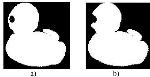
Fig.4: Applying the opening operator: a) the Original binary image b) the image opening.
