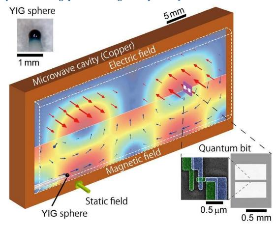
Illustration of magnet-qubit coupled system A magnet (ytterium iron garnet; YIG) and a superconducting qubit are placed with a separation of 4 cm. The electric field in the cavity interacts with the qubit, while the magnetic field interacts with the magnet. At an extremely low temperature of around -273 degrees centigrade, magnons, i.e., quanta of the fluctuations in the magnet, coherently couple with the qubit through the electromagnetic field of the cavity.
