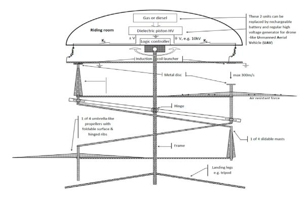
Fig. 3: quartet flapping umbrella propeller equipped aero-vehicle
