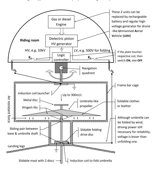
Fig. 1: Typical umbrella-like propeller for light duty aerial vehicle
