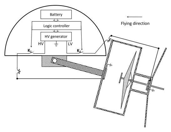
Fig. 2: UAV with umbrella-like propeller in flying
