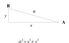
Clearly  $\sigma$  is not perpendicular to x or y. If the straight road from **A** to **B** slopes constantly either upward or downward then the truck also moves though a vertical distance (height) as it travels along the straight road from **A** to **B**. Then the distance s that the truck travels is given again by the Theorem of Pythagoras:
