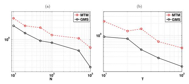
**Figure 8:** MSE (loglog-scale; averaged over  $10^3$  independent runs) obtained with the MTM and GMS algorithms (using the same proposal pdf and the same values of N and T) (a) as function of N with T=20 and (b) as function of T with N=100.
