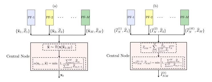
Figure 7: Graphical representation of Distributed Particle Metropolis-Hastings (DPMH) method, (a) for estimating a generic moment, or (b) for estimating of a specific moment of the target.
