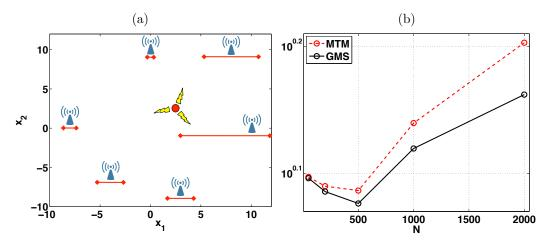
Figure 10: (a) Sensor network: the location of the sensors (antennas) and the target (circle) in the numerical example. The solid line represents the different unknown variances of the sensors. (b) MSE (log-scale) versus the number of candidates  $N \in \{50, 200, 500, 1000, 2000\}$  obtained by GMS and the corresponding MTM algorithm, keeping fixed the total number of evaluations  $E = NT = 10^4$  of the posterior pdf, so that  $T \in \{200, 50, 20, 10, 5\}$ .
