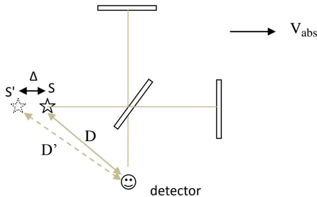
From the above diagram of the Michelson-Morley experiment, arranged for circular or straight parallel fringes, we see that the effect of absolute velocity is just to create an apparent change of the position of the light source relative to the detector, for absolute velocity  $V_{\text{abs}}$  directed to the right.
