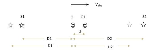
S1 and S2 are satellites, O represents control and monitoring station, O1 represents a GPS receiver. We assume that all clocks are perfectly synchronized, there is no relative motion between the satellites, the control and monitoring station and the GPS receiver, for simplicity. Our aim is to find the order of magnitude of error in position measurements caused by Earth's absolute motion ( 390 Km/s ).
