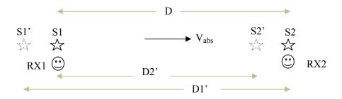
The operation of the clock is as follows: S1 emits a light pulse, then the detector RX2 detects the pulse, S2 transponds with another light pulse without delay, the detector RX1 detects the light
