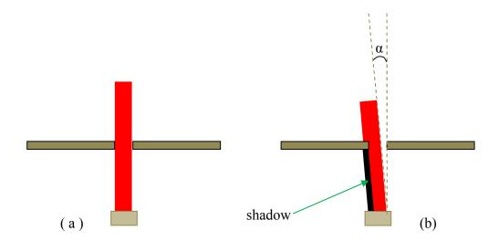
We can see that when the light is bent due to absolute motion, part of the light rays is blocked by the plate, creating a shadow and hence a decrease in intensity ( quantity of light per unit area ) of light falling on the photo detector. By measuring the voltage output of the photo detector, it is possible to observe variation of light intensity with variation in absolute velocity and with variation in orientation of line SD relative to the absolute velocity.
