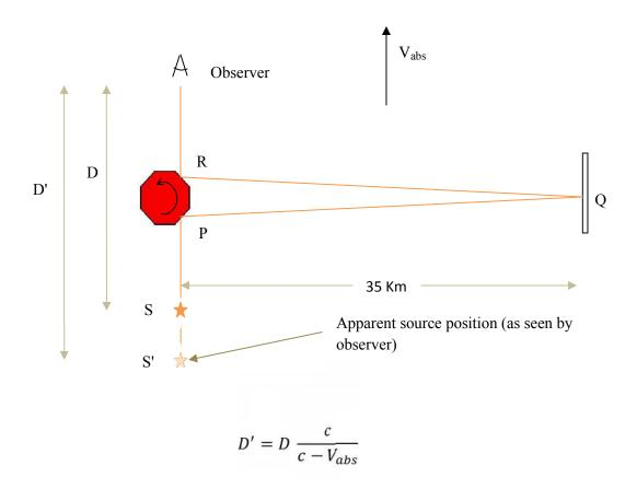
To clarify this interpretation, assume that sensors are put at points P, Q and R. Points P and R are points in space where the light is reflected from the rotating mirror, point Q is point on the distant mirror where the light is reflected. If a short light pulse is emitted by the source at time t = 0, then the light will be detected at points P, Q, and R, at times  $t_P$ ,  $t_Q$  and  $t_R$ , respectively.
