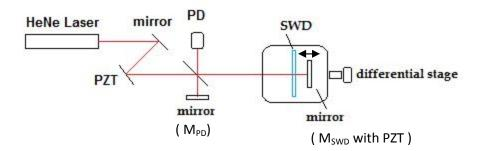
Doug Marett reported that he detected phase shift of the SWD voltage as the stage is moved, with the mirror  $M_{SWD}$  and the SWD detector co-moving with the stage. The  $M_{SWD}$  is also actuated with a triangle wave. How can movement of the stage create phase variation of the SWD voltage, with the mirror and the SWD sensor co-moving with the stage [20]?
