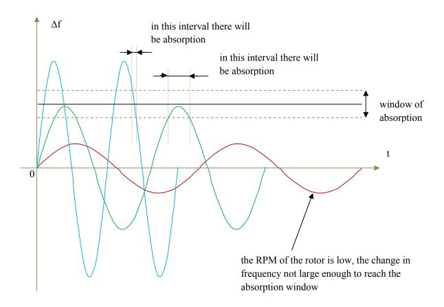
We assumed that there is no absorption at zero angular velocity, because the difference between the resonance frequencies of the source and the absorber is usually made slightly different.
