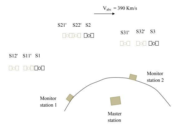
The control stations monitor the satellites from the signals they transmit and send the information to the master station, where the orbit and clock performance of each satellite is computed. These data are then uploaded to each satellite.
