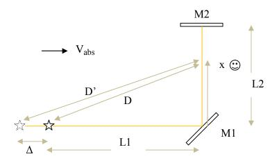
To analyze this problem, we first have to determine the apparent change in position ( $\Delta$ ) of the source as seen from point x, due to absolute motion. The time delay of the incident light will be:
