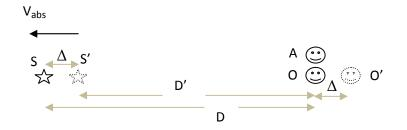
The apparent position of the source relative to the co-moving observer is determined from the following equations.
