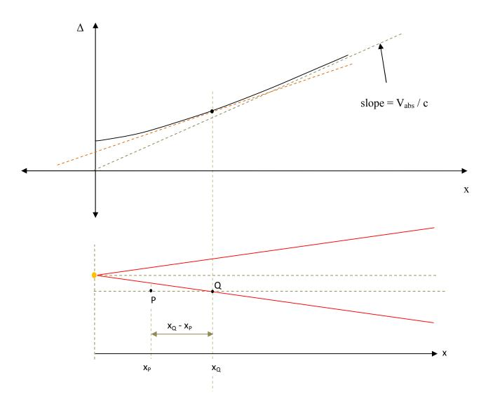
$$\frac{d\Delta}{dx} \text{ (at point P)} = \frac{d\Delta}{dx} \text{ (at point Q)}$$
