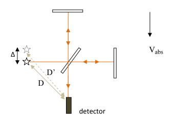
What is the effect of absolute velocity in this case? In the same way as above, we ask: what is the effect of actually, physically shifting the source position from S to S'? In this case also there may be a very small fringe shift because the two beams will be misaligned and will have slightly different path lengths. This may be why a very small fringe shift was always observed in conventional MM experiments.
