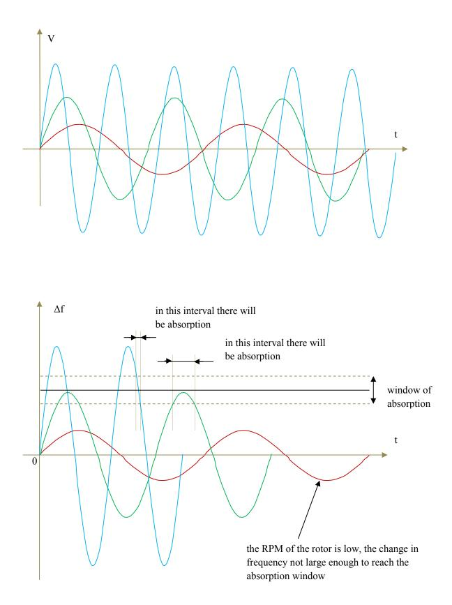
We assumed that there is no absorption at zero angular velocity, because the difference between the resonance frequencies of the source and the absorber is usually made slightly different.
