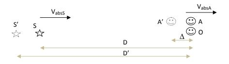
Suppose that the distance between a co-moving observer O ( the absolute velocity of O is the same as the absolute velocity of the source,  $V_{absS}$ ) and the source is D and that the moving observer (A) was at point A' relative to the source at the instant of light emission. Suppose that observer A is just passing through point A ( the same as point O ) at the instant that observer O detects the light. Therefore, observer A will also detect the light at that instant.
