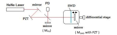
Doug Marett reported that he detected phase shift of the SWD voltage as the stage is moved, with the mirror  $M_{SWD}$  and the SWD detector co-moving with the stage. The  $M_{SWD}$  is also actuated with a triangle wave. How can movement of the stage create phase variation of the SWD voltage, with the mirror and the SWD sensor co-moving with the stage [20] ?
