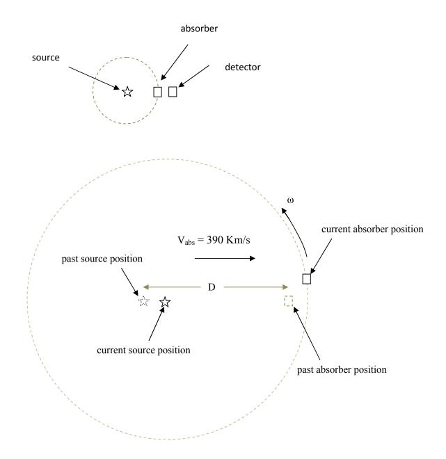
Why should we observe Doppler shift in the Mossbauer rotor experiment, as the source and detector are not in relative motion ? As stated in the last section, this is because the present observer ( at moment of detection) is moving relative to the past source (at moment of emission).
