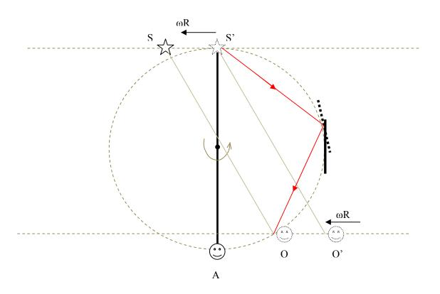
The problem is to determine the time delay of light between emission from the source S and detection by the moving observer A, after reflection from the mirror.
