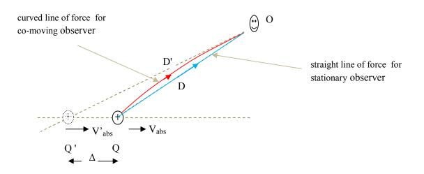
For the stationary observer, it is as if the electric field is rigidly carried by the moving charge, straight radial lines emanating from the charge. We explain this with AST as follows. For the stationary observer, the apparent change in position of the charge is exactly compensated for by the fact that the 'speed' of the electrostatic field will be *c relative* to the apparent charge Q'.
