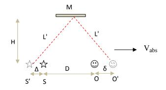
The time *T* elapsed for the light to travel from S', reflection at mirror, then arrive at O' is equal to the time taken for the observer to move from O to O'. The speed of light is *c* relative to the apparent source. We have to determine the speed of light *c'* in the dashed light ray, as seen in the absolute reference frame.  $\frac{2L'}{c'} = \frac{\delta}{V_{est}}$
