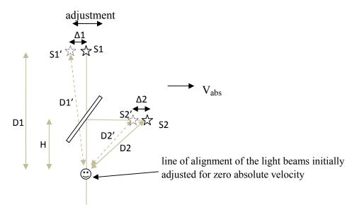
With zero absolute velocity, the two light beams arriving at the detector are adjusted to be aligned. Then, due to non zero absolute velocity, the two beams will be misaligned and a fringe shift will occur. The position of the source S1 may be adjusted (towards the right) until the two light beams are aligned again. The amount of adjustment of position of S1 required to align the two beams again can be used to determine the absolute velocity.
