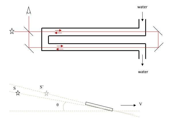
The Fizeau experiment is a stellar aberration phenomenon (Argo's water filled telescope experiment) with angle  $\theta = 0^0$  and  $\theta = 180^0$
