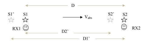
The operation of the clock is as follows: S1 emits a light pulse, then the detector RX2 detects the pulse, S2 transponds with another light pulse without delay, the detector RX1 detects the light pulse and S1 transponds without delay and so on. An electronic pulse counter can count the number of transmissions and hence a clock.
