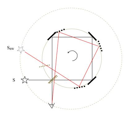
The position of the source apparently shifts towards when looking in the forward direction and away from the detector when looking in the backward direction. Therefore, a difference between path lengths of the backward light beam and the forward light beam arises resulting in a fringe shift. The apparent sources are at rest relative to the observer ( because the real source is at rest relative to the observer ) and the speed of light is constant relative to the apparent source.
