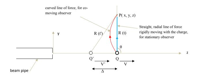
From the figure above, we can see that the maximum transverse electric field is detected at point P when the charge is physically at Q.
