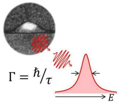
A single-photon source never emits two or more photons at the same time. Single photons are important in the field of quantum information technology where, for example, they are used in quantum computers. Alongside the brightness and robustness of the light source, the indistinguishability of the photons is especially crucial. In particular, this means that all photons must be the same color. Creating such a source of identical single photons has proven very difficult in the past.
