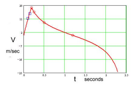
Figure-8, Measured projectile velocity (blue squares) verses theoretical results (red circles/line)
