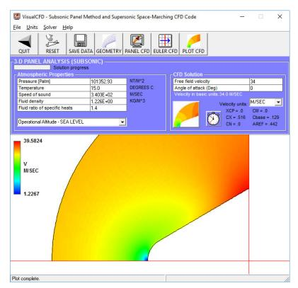
Figure-10, VisualCFD™ velocity contour plot. Cd = 0.516 and Cdbase = 0.129
