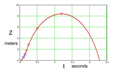
Figure-9, Measured projectile altitude (blue squares) verses theoretical results (red circles/line)
