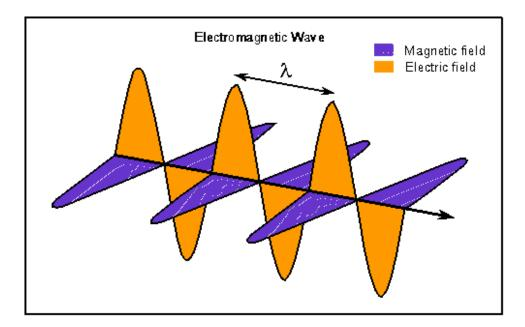
An electromagnetic wave showing electric and magnetic fields, and the wavelength  $(\lambda)$  which is the distance between crests of a wave.
