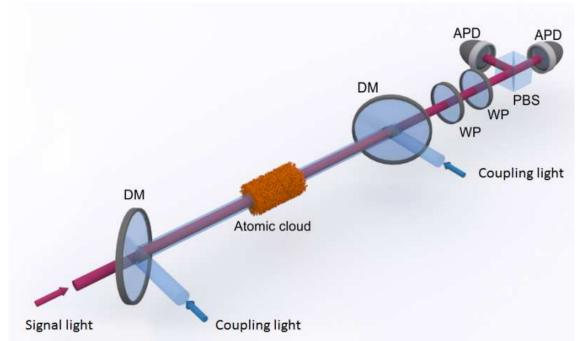
A cloud of cold atoms is illuminated with red signal light and blue coupling light. The light pulses are superimposed on dichroic mirrors (DM). With wave plates (WP), a polarizing beam splitter (PBS), and avalanche photodiodes (APD) the polarization of the transmitted signal light is determined.
