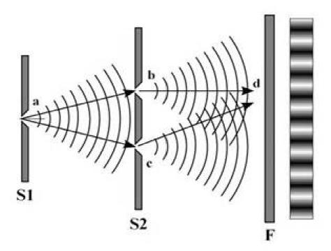
The above diagram shows the first plate (S1) with one slit producing a wave (a) propagating towards the second plate (S2) with two slits producing two individual waves (b & C) which produces an wave interference pattern (d) being displayed on the film screen (f). In the basic version the first plate (S1) is not used but coherent light such as a laser or a beam of electrons are fired directly at plate S2.
