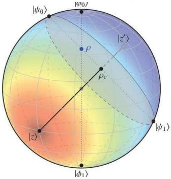
Entanglement on a sphere: This Bloch sphere shows entanglement for the one-root state p and its radial state pc. The color on the sphere corresponds to the value of the entanglement, which is determined by the distance from the root state z, the point at which there is no entanglement. The closer to z, the less the entanglement (red); the further from z, the greater the entanglement (blue). Credit: Regula and Adesso. ©2016 American Physical Society
