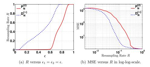
Figure 5: (a) Resampling Rate R as function of  $\epsilon_1 = \epsilon_2 = \epsilon$  for  $P_N^{(2)}$  (solid line) and  $D_N^{(\infty)}$  (dashed line). b Mean Square Error (MSE) as function of the resampling Rate R for  $P_N^{(2)}$  (solid line) and  $D_N^{(\infty)}$  (dashed line), in log-log-scale (N = 1000 and T = 3000).
