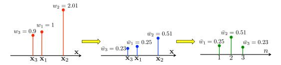
Figure 1: Graphical representation of the loss of statistical information normalizing the weights and removing the positions of the particles (N=3).
