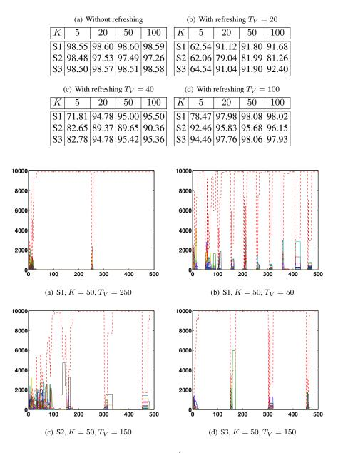
**Fig. 5**: Number of particles  $M_{k,t}$  (with K = 50 filters and  $N = 10^5$ ) as function of the iterations t, in one specific run. The number of particles of the filter corresponding to the true model is depicted with a dashed line. Figures (a) and (b) correspond to the setup S1 and  $T_V = 50, 150$ , respectively; Figures (c) and (d) correspond to the setup S2 and S3 with  $T_V = 150$ , in both cases.
