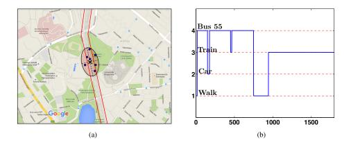
Fig. 7: (a) Example of generation of particles (shown as circles) using the dynamic model of type in Eq. (53). (b) Detection of transition between Bus 55, Walk and Train (MAP estimation) at the Helsinki central railway station, considering 4 possible modalities with real data ( $T \approx 1900$  sec and  $T_V = 150$  sec).
