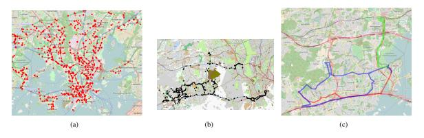
**Fig. 6**: (a) All bus stops in Helsinki region (left). (b) All intersections crossed during a 10-day period by one participant. (c) A small section of trajectories labeled under different transportation modes. Blue is car, red is bus, and green is cycling.
