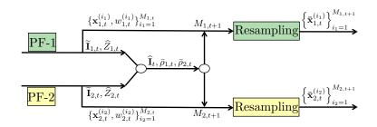
Fig. 2: Another graphical representation of the MAPF scheme, with K = 2 parallel particle filters. A fusion center returns,  $\hat{\mathbf{I}}_t$ ,  $\bar{\rho}_{k,t}$ , and the numbers of particles  $M_{k,t+1}$ , k = 1, 2, of the next iterations. Then, the resampling steps are performed separately.
