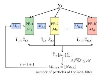
Fig. 1: Graphical overview of the MAPF scheme in Table 2 for approximating the MMSE estimator  $\hat{\mathbf{I}}_t$  and the posterior of each model given the observed data. Note that  $\widehat{ESS}$  in Eq. (39) takes into account the (normalized) weights  $\bar{\gamma}_{k,t}^{(i_k)} = \bar{w}_{k,t}^{(i_k)} \bar{\rho}_{k,t}$ , for all  $i_k$  and k.
