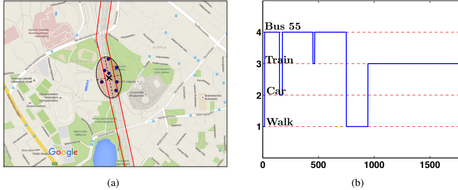
Fig. 7: (a) Example of generation of particles (shown as circles) using the dynamic model of type in Eq. (54). (b) Detection of transition between Bus 55, Walk and Train (MAP estimation) at the Helsinki central railway station, considering 4 possible modalities with real data ( T \approx 1900 sec and T_V = 150 sec).
