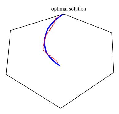
Figure 1: The interior of the polygon comprises all points (x, y, s) satisfying Ax = b and  $A^Ty + s = c$ , x > 0, and s > 0. The blue (bold) line consists of all points in this polygon with  $x_i s_i = \mu$  for all *i* and some  $\mu > 0$ . The optimal solution is a vertex of the polygon corresponding to  $x_i s_i = 0$  for all *i*. The red (dashed) line illustrates the steps of the algorithm. It follows the blue (bold) line in discrete steps.
