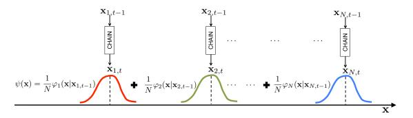
Fig. 2. A graphical representation of the mixture-based strategy. The mixture  $\psi(\mathbf{x})$  is formed by N components,  $\varphi_n(\mathbf{x}|\mathbf{x}_{n,t})$ , where  $\mathbf{x}_{n,t} \in \mathcal{P}_t$  plays the role of location parameter.
