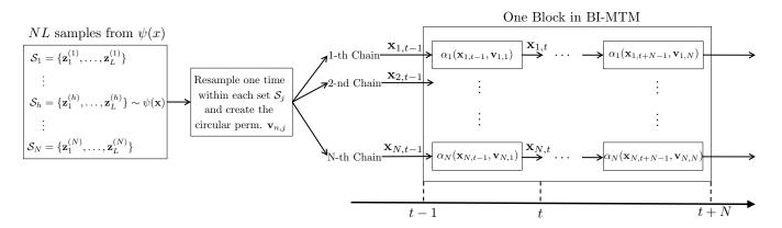
Fig. 4. A graphical representation of one block within the BI-MTM technique, described in Table 6. One specific transition of one MTM chain is represented with the probability  $\alpha_n(\mathbf{x}_{n,t-1}, \mathbf{v}_{n,j})$ , showing the two possible future states at the *t*-th iteration, of the *n*-th chain. One block is formed by *N* transitions.
