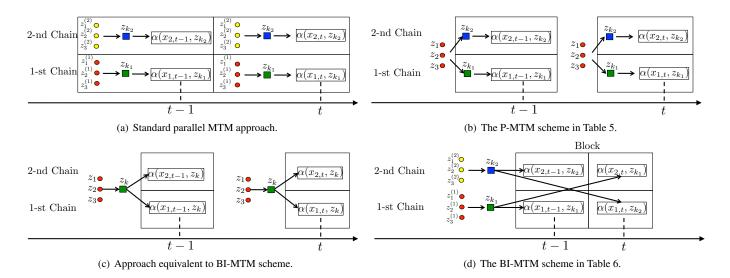
Fig. 8. A graphical representation of the several parallel MTM schemes with N = 2 chains and L = 3 tries. The BI-MTM scheme in (d) requires only 6 evaluations of the target pdf and 2 multinomial sampling steps considering two iterations, t - 1 and t.
