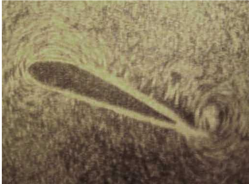
Fig.2. Origination of the circulation around a moving airplane wing. The vortices at the rear edge trigger a motion of the air around the wing according to the angular momentum conservation law.
