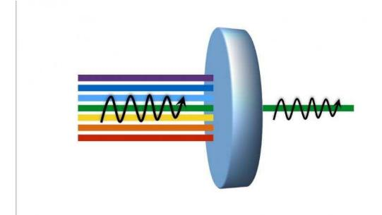
A quantum emitter (represented as the blue disk) interacts with an electromagnetic field. Physicists have learned that dipole-dipole interactions in said quantum emitters can be manipulated to make opaque objects look transparent (Image Credit: Puthumpally-Joseph, et al, American Physical Society)
