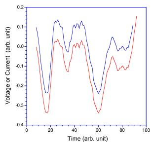
**Figure 3.** Computer generated example to illustrate how can a DC shift distinguish two strongly correlated noises by using a very shot sample. If the DC shift is greater than the stochastic difference between the time functions then a single-time measurement is enough to distinguish the two noises and the bit situations in KLJN.
