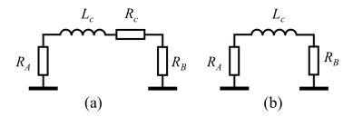
Fig. 2. Lumped impedance-components-based model of a cable at low frequencies for analyzing voltage drop along the cable and phase shift in the limit  $f \ll f_{min}$ . Part (a) represents a cable with loss (cable inductance and resistance are designated  $L_c$  and  $R_c$ , respectively), and part (b) represents a lossless cable.
