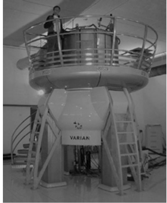
Fig.5 - A 0.9 \text{ GHz} , 21.1 \text{ T} NMR spectrometer at HWB-NMR, Birmingham, UK.
