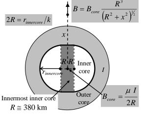
Fig. 1 – Similarity between the magnetic field produced by a toroid and the Earth's magnetic field.
