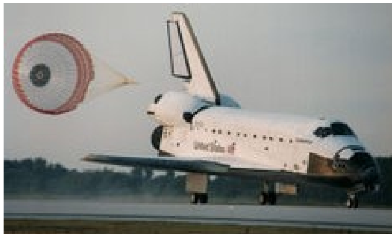
Figure 4-3. Endeavour deploys drag chute after touch-down.
