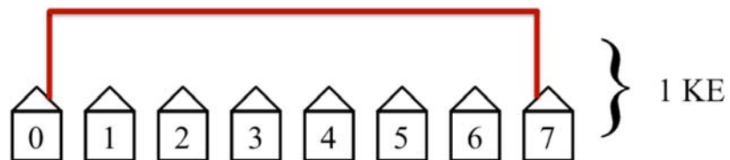
Figure 14. The seventh and last step. This step is not efficient but only requires one KE since there is only one such pair of hosts.
