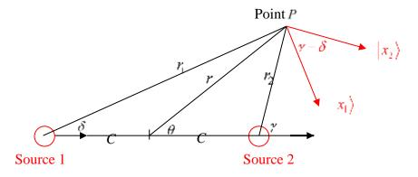
**Figure 3.5. 2** Two sources 2C apart, both with  $\beta_{nk}^2 \times (m = +2)$  states along the joining line,  $\delta \& \gamma$  are the respective angles to P,  $r_1 \& r_2$  are the respective distances to point P.
