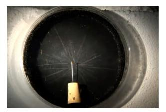
Fig. 9: the Wilson Cloud Chamber (intense cosmic radiation at high altitude condenses water clouds).
