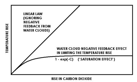
**Fig. 10:** negative feedback equation gives "saturation effect" law,  $T \sim 1 - e^{-C}$  where C is relative concentration of carbon dioxide, rather than a linear law. In other words, negative feedback means that large amounts of  $CO_2$  are opposed by increasing cloud cover "global dimming," like a thermostat. The origins of this are in Jim Lovelock's Gaia theory:
