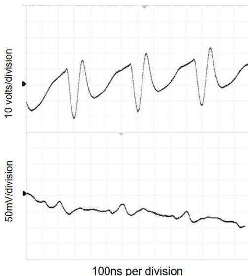
Fig. 8 Transmitter antenna vs receiver antenna voltages.
