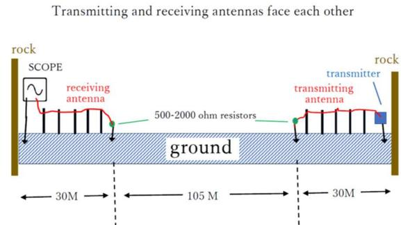
Fig. 4 Transmitting and receiving antennas face each other
