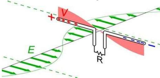
Fig. 1 Radio waves emitted by a resonating dipole antenna
