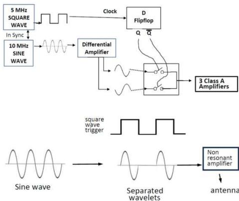
Fig. 3 Transmitter block diagram.
