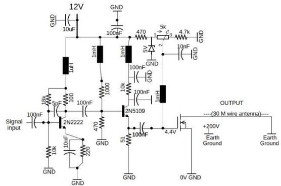
Fig. 11 3 transistor class A amplifier.
