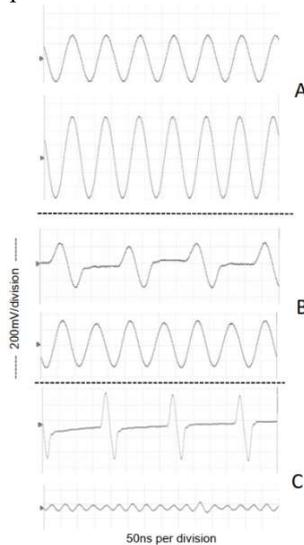
Fig. 2 Effect of bandpass filter on single, multiple pulses.
