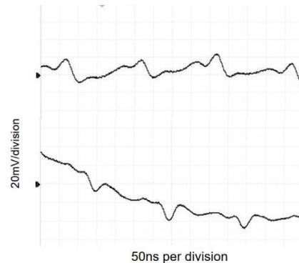
Fig. 6 Received signals, no ground on transmitter.
