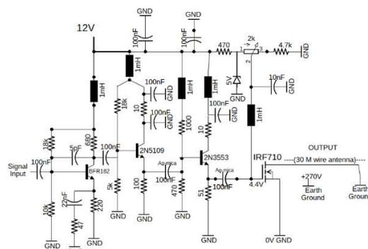
Fig. 12 4 transistor class A amplifier
