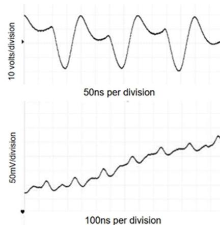
Fig. 7 Transmitter antenna vs receiver antenna voltages.
