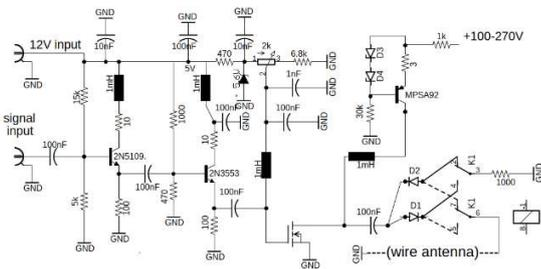
Fig. 9 AC vs DC transmitter circuit.
