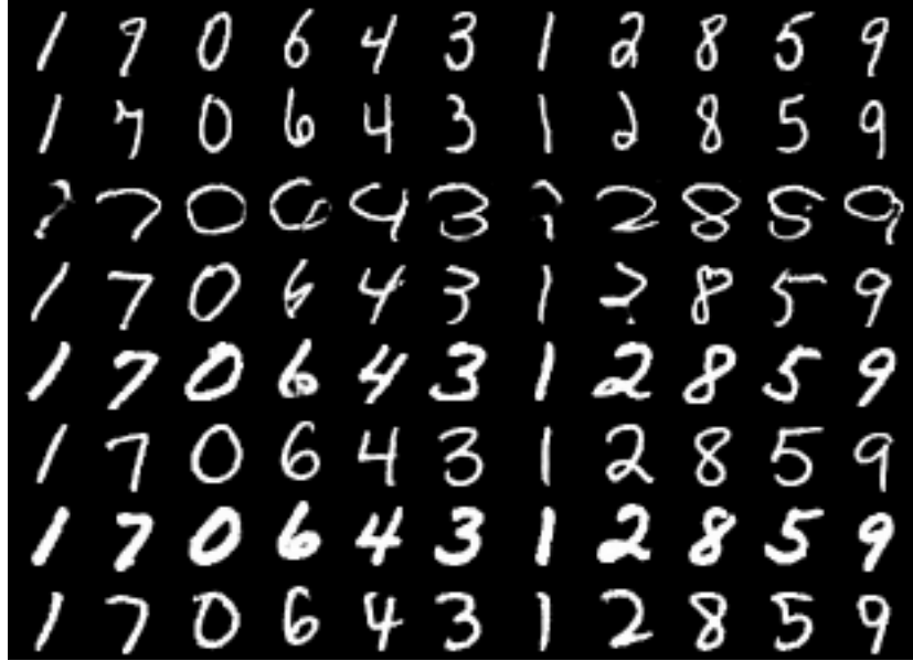
Figure 9: MNIST generated data with \lambda_{creg} = 50 . Each row has the same continuous latent code, and each column has the same categorical latent code. Out of d_c categories, those with a probability less than 1% were excluded. The probabilities for each category are [0.0434, 0.1054, 0.1017, 0.1003, 0.0985, 0.1046, 0.0656, 0.0998, 0.0978, 0.0879, 0.0951]. FID: 2.7041, precision: 0.8206, recall: 0.6687.
