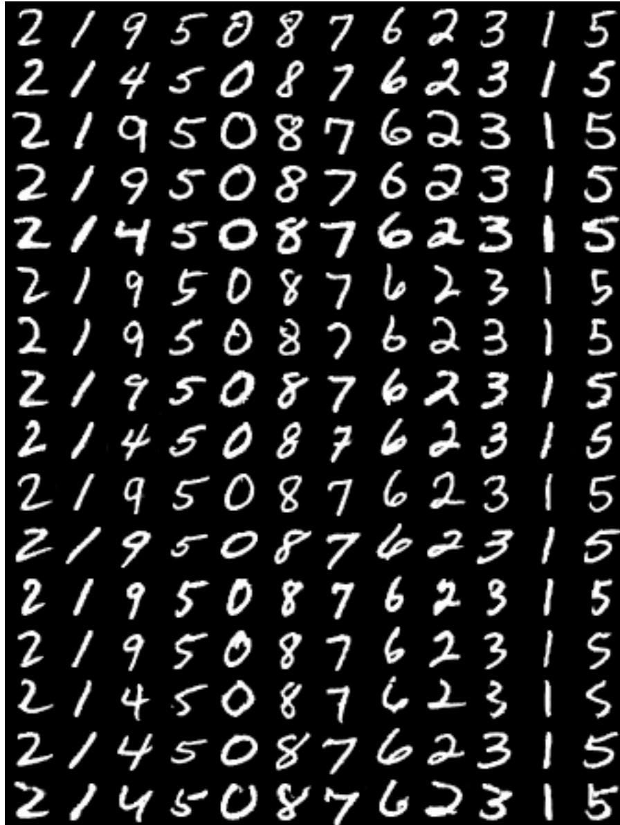
Figure 6: MNIST generated data with \lambda_{creg} = 20 . Each row has the same continuous latent code, and each column has the same categorical latent code. Out of d_c categories, those with a probability less than 1% were excluded. The probabilities for each category are [0.0268, 0.0456, 0.1936, 0.0404, 0.0992, 0.0970, 0.1061, 0.0993, 0.0694, 0.1037, 0.0673, 0.0481]. The entropy of categorical latent distribution is 2.3776. FID: 2.1096, precision: 0.8104, recall: 0.7033.
