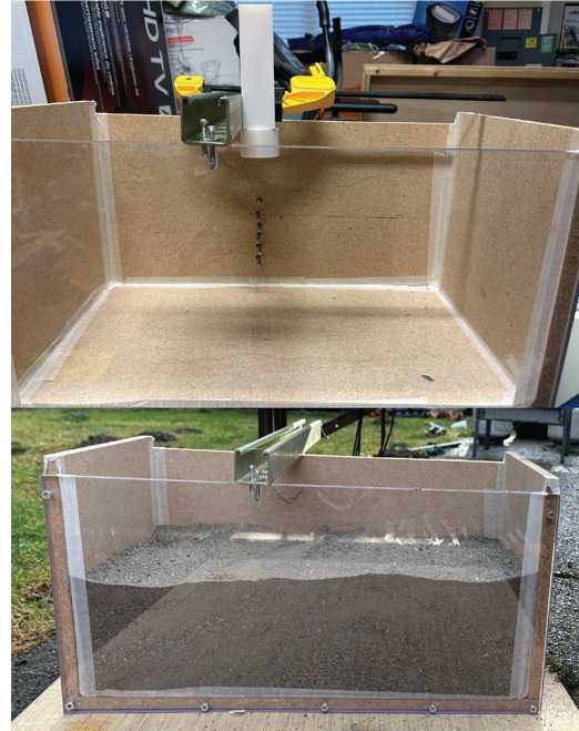
Figure 1: Static launch rig with temperature probes slightly exposed on the back wall in the middle of the rig. The steel beam connecting the polycarbonate visibility panel and the wooden back wall is the mounting beam for the rocket motor.
