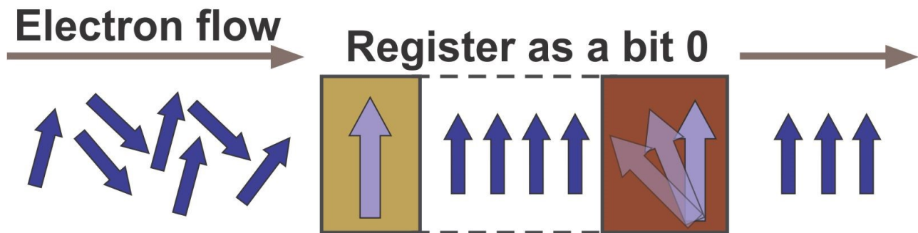
Figure 5: Polarization fields aligning spins of the electron flow. Magnetic resistance on tunneling, an electric current flows easily, through the two magnetic configurations that lead to spins with the same sense and showing resistance when opposite spins senses result from differently oriented magnets.
