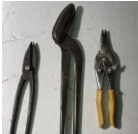
Fig.1. Curved (in the middle) and straight (left and right) claws of the cutter
