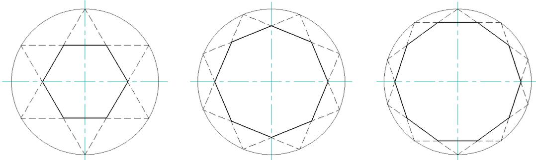
In this second case I have always started from polygons with an even number of sides, and the minimum number of sides is 6.
