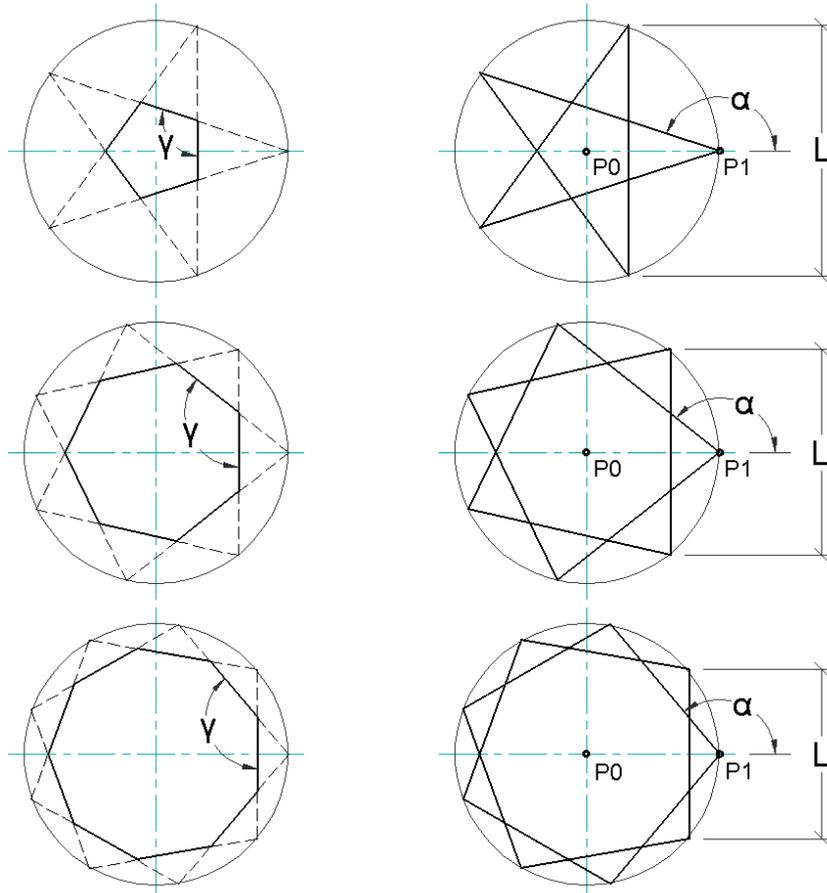
So to conclude, this last type of stars can be made from a polygonal that starting from a point (P1) with a number of segments equal to the reference polygon, after having completed two turns around the origin (P0), returns to (P1) having made a closed figure in the shape of a star.
