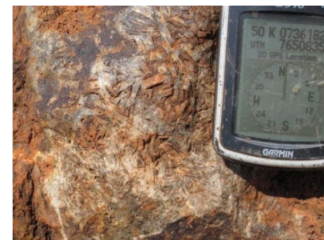
33C : Bernts Gossan : Siliceous gossan with breccia textures and ex-barite veins.
