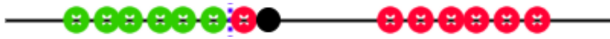
Figure 2.5: A margin classifier being affected by an outlier (the red circle close to the green circles) causes the new black sample to be classified as red despite being closer to the green group [Gun20]
