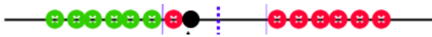
Figure 2.7: The new black sample will be classified as green because of the support vector being calculated to be between the majority of the elements of each class [Gun20]
