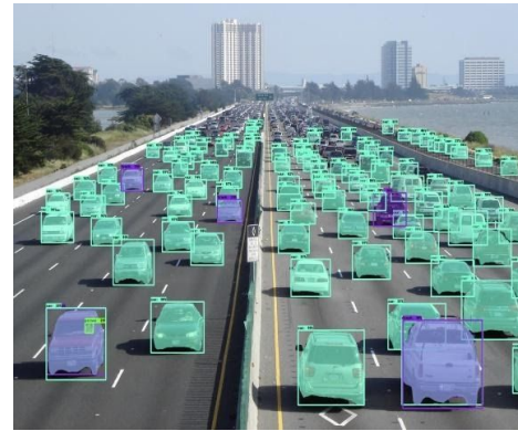
Fig.7: Visualization of vehicle’s detection results using Mask R-CNN Image Segmentation Model
