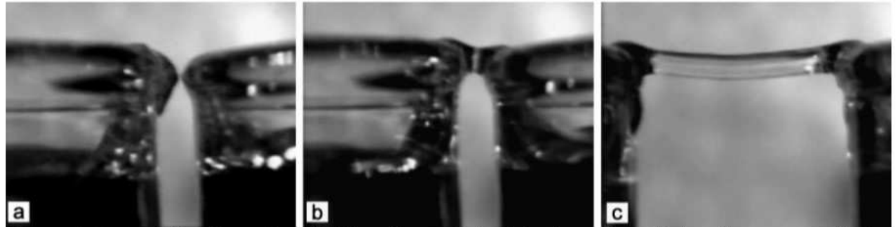
Figure 1. Water bridge formation: (a) Rise of water in both beakers after a high voltage was applied and a first ignition spark was observed , (b) spontaneous formation of a connection which remains stable after (c) pulling the beakers apart .
