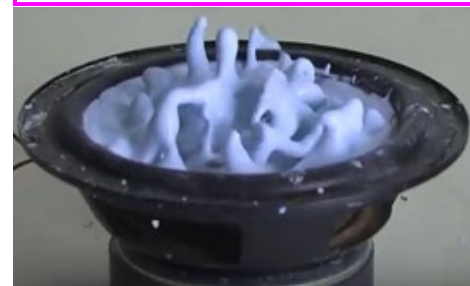
Movie_12 : Non-Newtonian Fluid on a Speaker Cone ( → Corn starch, a shear thickening non-newtonian fluid was used )
