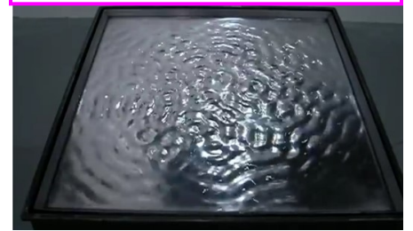
Movie_4 : Sound monolith resonance pattern – water ( excited by sound )
