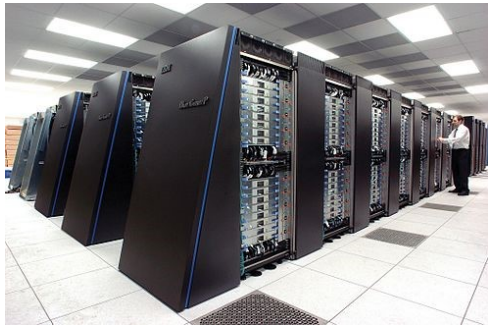
The IBM Blue Gene/P supercomputer "Intrepid" at Argonne National Laboratory runs 164,000 processor cores using normal data center air conditioning, grouped in 40 racks/cabinets connected by a high-speed 3-D torus network.
