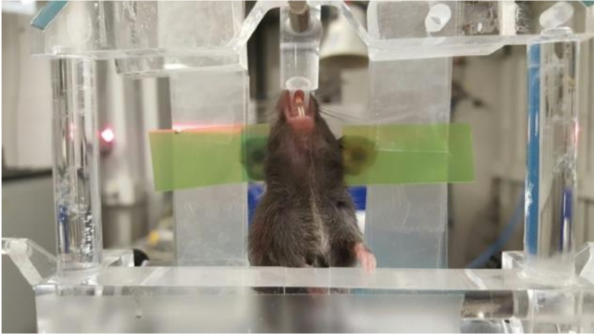
Irradiation set-up showing radiochromic film placed behind the irradiated ear. (Courtesy: Marine Potez)
