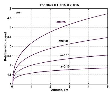
**Fig. 7.** Relative wind speed versus altitude for  $V_o = 6$  m/s,  $H_o = 10$  m/s.
