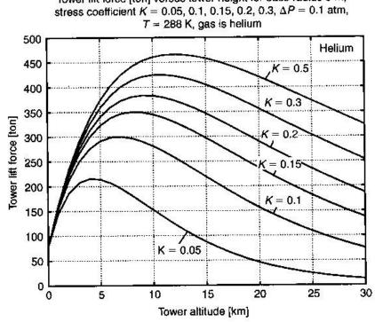
Tower lift force [ton] versus tower height for base radius 5 m,
