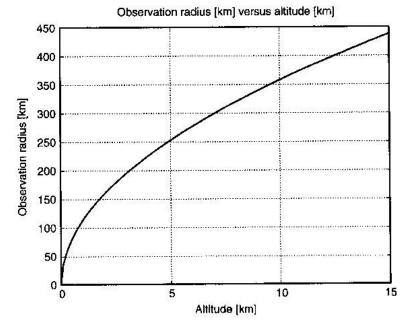
Fig. 4.4. Observation radius for altitudes up to 15 km
