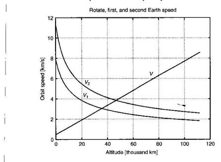
Fig. 1.18. Rotate, first, and second Earth speed [km/s] via altitude [thousand km].
