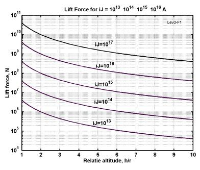
**Figure 5.** Lift force of AB-Levitron space station versus the relative altitude for a product of the electric currencies the superconductivity ground and station rings and for the optimal ground ring.  $\overline{h} = h/r$ , *h* is station altitude, *r* is radius of top ring.
