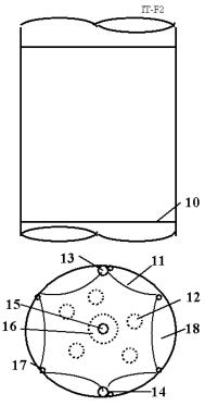
Fig. 4.2. Section of inflatable tower. Notations: 10 – horizontal film partitions; 11 – light second film (internal cover); 12 – air balls; 13 – entrance line of compression air and pressure control; 14 – exit line of air and control; 15 – control laser beam; 16 – sensors of laser beam location; 17 – control cables and devices; 18 – section volume.
