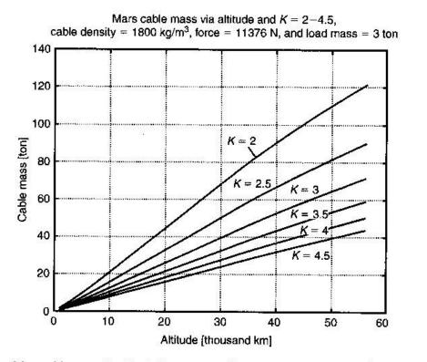
Fig. 1.24. Mars cable mass via altitude [thousand km], a cable density 1800 kg/m<sup>3</sup> and a load mass of 3 ton.
