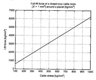
Fig. 3.14. Full lift force of the closed-loop cable circle rotated around a planet.
