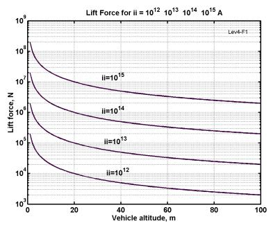
**Figure 6.** Lift force [N/m] of the 1 meter AB-Levitron multipath highway versus the train (vehicle) altitude for a product (*ii*) of the electric currencies of the superconductivity ground and vehicle rings.
