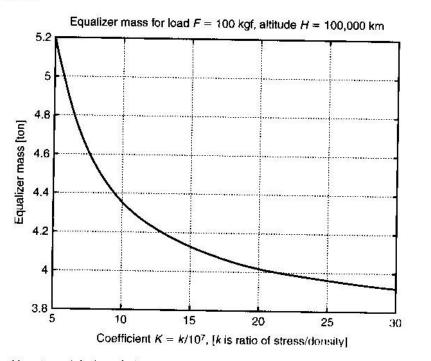
**Fig. 1.14.** Counterweight [tons] via altitude [thousand km] for ground force 100 kgl (at Earth's surface) for K = 5 (0.11) is centrifugal force without additional force which supports the cable of equal stress.)
