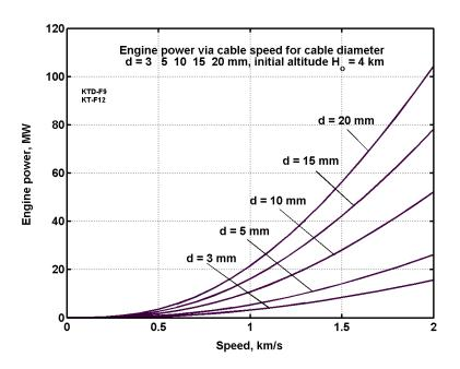
Fig. 5.12. Engine power via cable speed 0–2 km/s for different cable diameter.
