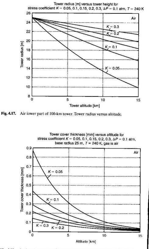
Fig. 4.18. Air lower part of 100-km tower. Tower cover thickness versus nititude.
