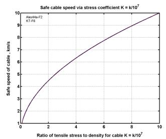
Fig. 5.6. Safe cable speed via relative stress coefficient K = 1-10.
