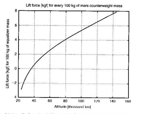
Fig. 1.25. Lift force [kgf] via aititude [thousand km] for every 100 kg of Mars equalizer mass.
