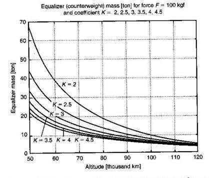
**Fig. 1.11.** Counterweight (equalizer mass) [tons] via altitude [thousand km] for ground force 100 kgf (at Earth's surface) for K = 2-4.5. (It is centrifugal force without additional force, which supports the cable of equal stress.)
