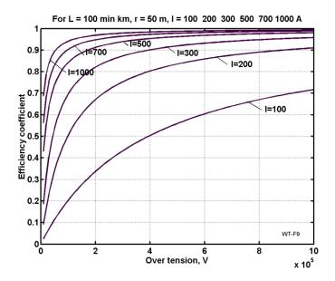
Figure 13. Coefficient efficiency of the electric transfer via over electric tension for different electric currency, distance 100 millions of kilometers and radius of plasma cable 50 m.
