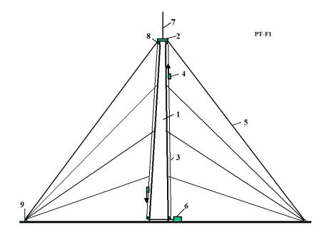
Fig. 4.1. Inflatable tower of height 3 km (10,000 ft). Notations: 1 – Inflatable column of radius 5 m; 2 – observation desk; 3 – load cable elevators; 4 – passenger cabin; 5 – expansions; 6 – engine; 7 – radio and TV antenna; 8 – rollers of cable transport system; 9 – stability control.
