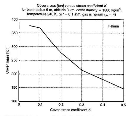
Fig. 4.14. Cover mass versus stress coefficient for the 30-km helium tower.
