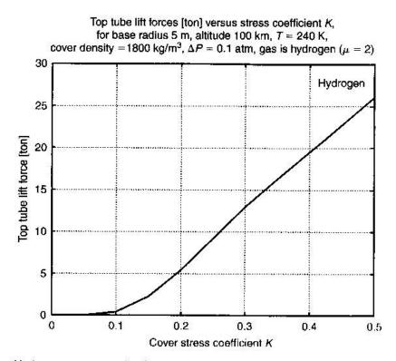
Fig. 4.26. Hydrogen top part of 100-km tower. Tower top lift force.
