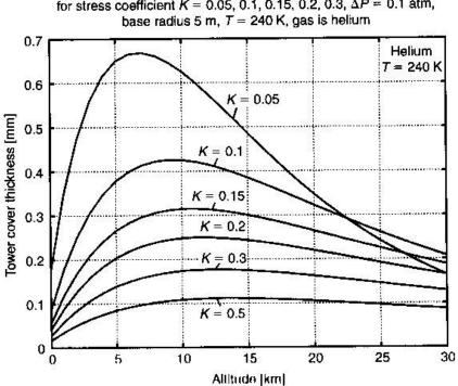
Tower cover thickness [mm] versus altitude for stress coefficient  $K = 0.05, 0.1, 0.15, 0.2, 0.3, \Delta P = 0.1$  atm, base radius 5 m, T = 240 K, gas is helium
