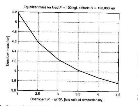
**Fig. 1.13.** Counterweight [tons] via altitude [thousand km] for ground force 100 kgf (at Earth's surface) for K = 2-4.5. (It is centrifugal force without additional force, which supports the cable of equal stress.)
