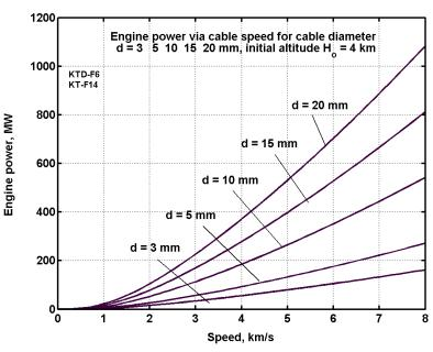
Fig. 5.14. Engine power via cable speed 2-8 km/s for different cable diameter.
