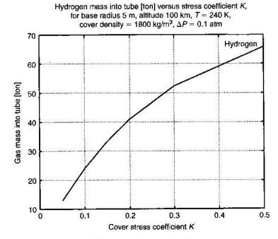
Fig. 4.27. Hydrogen top part of 100-km tower. Required hydrogen mass.
