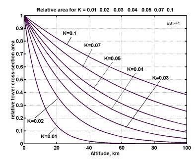
Figure 3. Relative tower cross-section aria versus tower altitude (up 100 km) and pressure strong coefficient.
