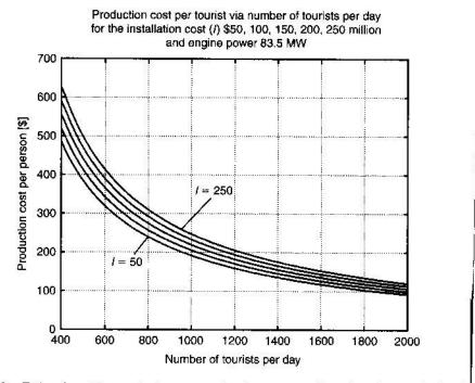
**Fig. 3.19.** Estimation of the production cost per tourist versus number of tourists per day for the installation cost US \$ (in million): 50, 100, 150, 200, and 250 and engine power 83.5 MW.
