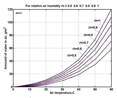
Fig. 4. Amount of water in 1 m<sup>3</sup> of air versus air temperature and relative humidity (rh).  $t_1 = 0$  °C.
