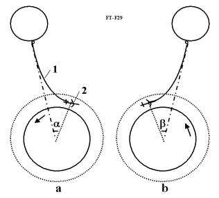
Fig. 1.31. Temporary landing of the Moon aircraft on the Earth's surface for loading. a-landing, b- take-off.
