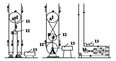
Fig. 1.4. Two mechanisms for changing the rope length in the Transport System (They are same for the space station). Notations: 11 - the rope which is connected axis A, B. This rope can change its length (the distance AB); 12 - additional rollers.
