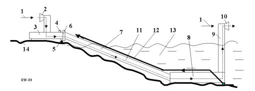
Fig.3. Sea extractor freshwater from atmosphere. Notation: 1 - wind, 2 - air entrance, 3 - solar air heater, 4 injector of sea water, 5 - collector of superfluous sea water, 6 - air ventilator, 7 - air tube, 8 - radiator (heat exchanger), 9 - exit air tube, 10 - exit air flow, 11 - air flow, 12 - freshwater line, 13 - sea, 14 - ground.
