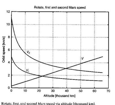
; 1.28. Rotate, first, and second Mars speed via altitude [thousand km].
