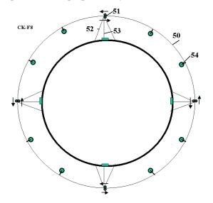
**Fig. 3.8.** Cable circle around the Earth for 8-10 space objects. Notations are: 50 – double circle, 51 – drive stations, 52 – guide cable, 53 – energy transport system, 54 – space station.
