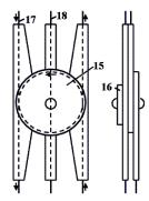
Fig. 1.5. Roller of Space Transport System. Notations: 15 – roller, 16 – control; 17 – transport system cable; 18 – main cable.
