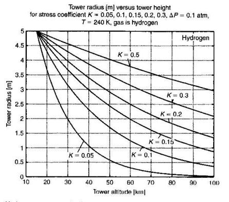
Fig. 4.22. Hydrogen top part of 100-km tower. Tower radius versus attitude.
