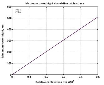
Fig. 5.7. Maximum tower height via relative cable stress.
