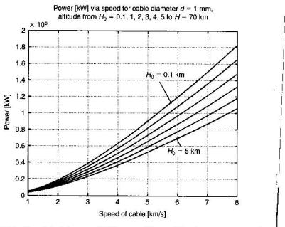
Fig. 3.18. Estimation of the drive power [kW] versus cable speed [km/s] and initial altitude [km] for a double semi-circle keeper.
