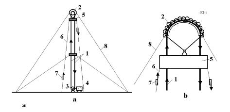
Fig.5. Offered kinetic tower: 1 – mobile closed loop cable, 2 – top roller of the tower, 3 – bottom roller of the tower, 4 – engine, 5 – space station, 6 – elevator, 7 – load cabin, 8 – tensile element (stabilizing rope).
