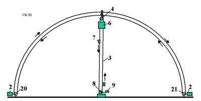
Fig. 3.2. Semi-circle launcher (space station keeper) and transport system. Notation is the same with Fig. 3.1 with the edditional 20 and 21 - rollers. The semi-circle is the same (see right side of Fig. 3.4).
