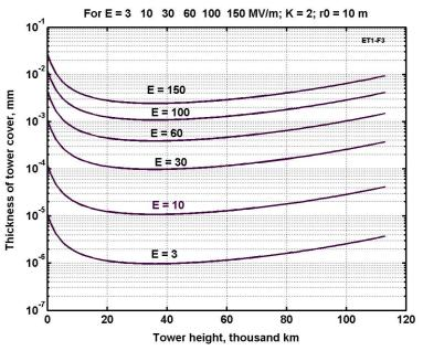
Fig. 5. Thickness of tower cover versus tower height for different electric intensity and base radius  $r_o = 10$  m and strength coefficient K = 2.
