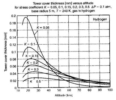
Pie. 4.34. Hydrogen top part of 100-km tower, lower cover thickness.
