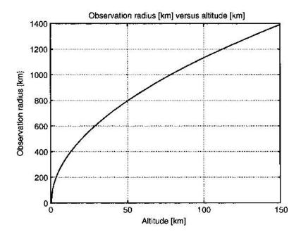
Fig. 4.5. Observation radius for altitudes up to 150 km.
