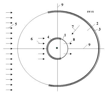
Fig.2. Inflatable extractor freshwater from atmosphere (top view). *Notation*: 1 - vertical inflatable tube, 2 - solar heater (optional), 3 - wind leafs of solar heat, 4 - wind leafs of air exit, 5 - wind at ground, 6 - wind at altitude, 7 - solar radiation, 8 - exit tube air flow, 9 - tube support cable.
