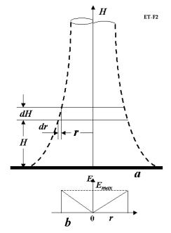
Fig. 2. (a) For explanation of theory optimal cross-section area of the electrostatic AB tower. (b) graph of electric intensity into tower
