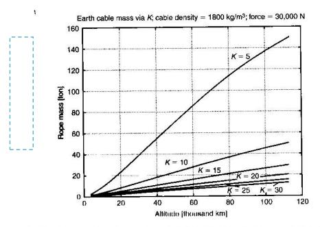
**The L9.** Cable mass [tons] via counterweight altitude for Farth's surface force of Vion, cable **instance kg/m<sup>3</sup>**, and K = 5-30.
