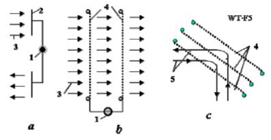
Figure 3. Getting the plasma currency energy from plasma cable. a - getting by two thin conducting films; b - getting two nets which brake the electric current flux; c - plasma reflector. Notations: 1 - spaceship or space station, 2 - set (films) for collect (emit) the charged particles, 3 - plasma cable, 4 - electrostatic nets.
