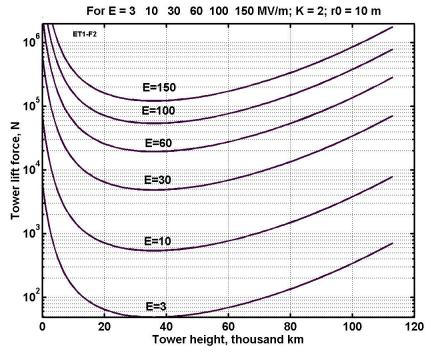
The computation lift force via altitude for different *E*, K = 2 and base  $r_0 = 10$  m is presented in fig.4.
