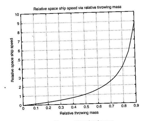
Fig. 3.15. Relative speed of space ship versus relative throwing mass.
