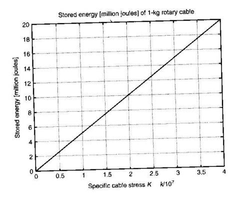
Fig. 3.16. Storage energy of 1 kg of the cable
