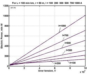
Figure 12. Transferred electric power (millions W) via voltage over minimum electric tension (see requested minimum tension in Figure10) for different electric currency, distance 100 millions of kilometers and radius of plasma cable 50 m.
