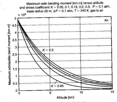
Fig. 4.19. Air lower part of 100-km tower. Maximum safe bending moment.
