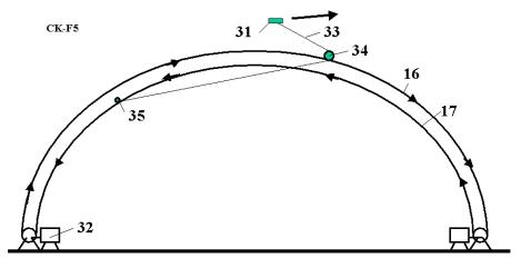
**Fig. 3.5.** Launching a load into space with a triple circle rope speed using the double semi-circle. Notations are: 31 – space probe, 32 – engine, 33 – launch cable, 34 – roller, 35 – connection point of the launch cable, 16, 17 – semicircle.
