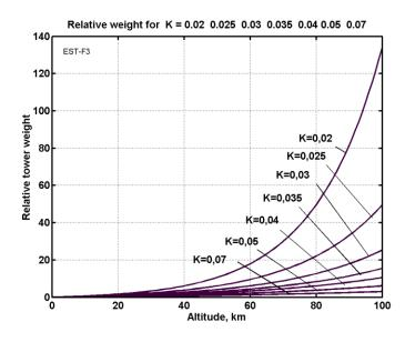
Figure 4. Relative tower mass for height H = 100 km versus pressure stress coefficient K.
