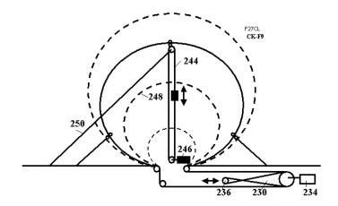
**Fig. 3.9.** System for changing the radius of the circle circle. Notations are: 230 – system for radius control, 234 – engine, 236 – mobile tackle block, 244 – transport system, 246 – engine, 248 – circle, 250 – guide cable.
