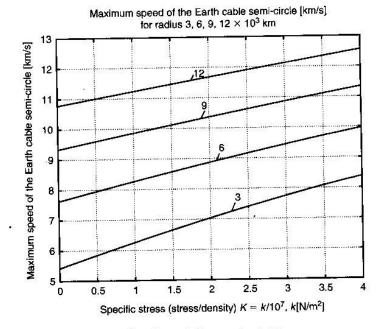
Fig. 3.13. Maximum speed of a closed-loop circle around a planet.
