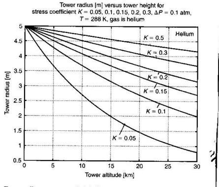
Fig. 4.11. Tower radius versus tower height for the 30-km helium tower.
