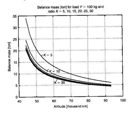
Fig. 1.12. Counterweight [tons] via ultitude [thousand kin] for ground force 100 kgf (at Earth's surface) for K = S = 30. (It is centrifugal force without additional force, which supports the cable of **stress.**)
