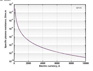
Figure 10. Specific plasma resistance  $\Omega$ .m of equilibrium plasma cable versus electric currency, A.
