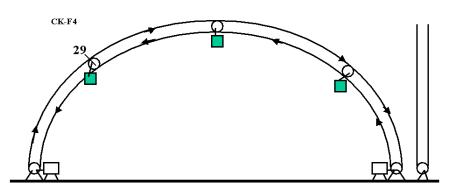
Fig. 3.4. Double semi-circle with opposed speeds for delivery of load to another semi-circle end. 29 -Roller.
