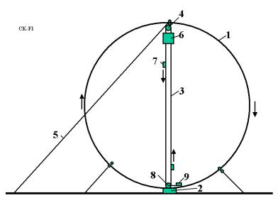
Fig. 3.1. Circle launcher (space station keeper) and space transport system. Notations are: 1 – cable circle, 2 – main engine, 3 – transport system, 4 – top roller, 5 – additional cable, 6 – the load (space station), 7 – mobile cabin, 8 – lower roller, 9 – engine of the transport system.
