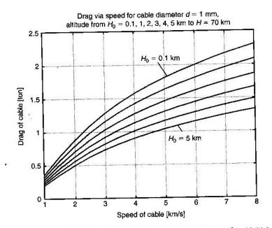
**Fig. 3.17.** Estimation of the friction air drag [ton] versus cable speed [km/s] and initial altitude [km] for a double semi-circle keeper.
