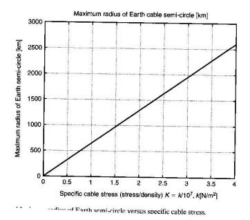
Fig. 3.12. Maximum radios of the Earth semi-circle versus specific cable stress
