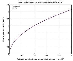
Fig. 5.5. Safe cable speed via stress coefficient K = 0-1.
