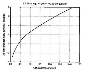
Fig. 1.10. Lift force [kgf] via altitude [thousand km] for every 100 kg of a counterweight (equalizer).
